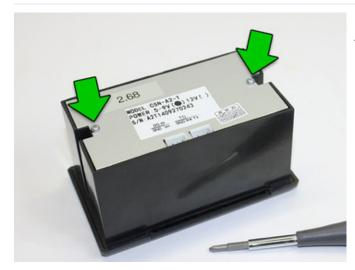
Unplug all cables, turn the printer over and remove the two small Phillips screws.
