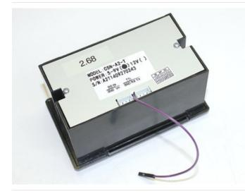
Screw the controller board back in place (check that neither of the cables has come unseated), routing the DTR wire around between the two sockets, then screw the back on.
