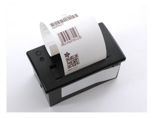
Add a mini printer to any microcontroller project with this very cute thermal printer. Also known as receipt printers, they're what you see at the ATM or grocery store. Now you can embed a little printer of your own into an enclosure. This printer is ideal for interfacing with a microcontroller, you simply need a 3.3V to 5V TTL serial output from your microcontroller to print text, barcodes, bitmap graphics, even a QR code!
