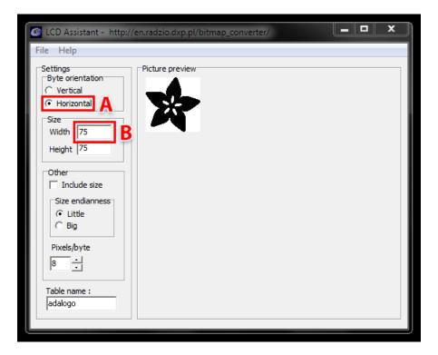
First, in the "Byte orientation" section of the settings, select "Horizontal" (item A in the image above).
