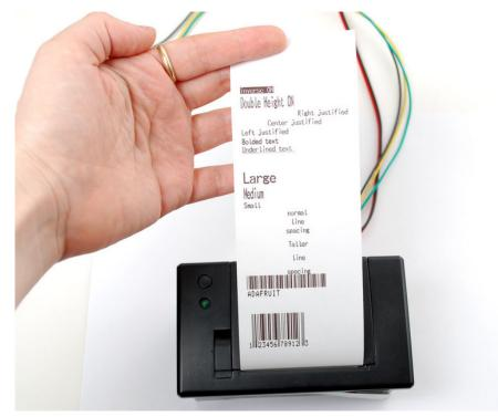
The thermal printer has a few handy things it can do, most of which are in the **A\_printertest** sketch. These are shown in the image above. In order, starting from the top:
