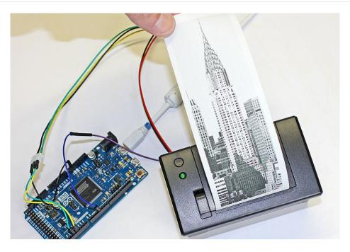
The printBitmap() function can output images from an open stream or stored in PROGMEM (flash memory)...as explained on the "Printing Bitmaps" page.
