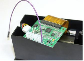
Solder the wire to the DTR pad. Top, bottom, doesn't matter...it's right up against the serial connection plug, so use whatever path works best for you, there's ample room for routing the wire around either way.
