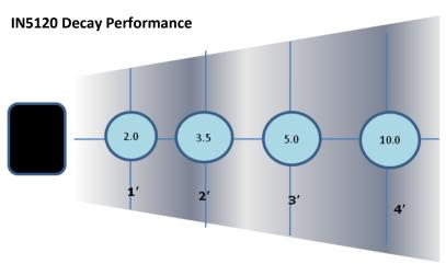
Testing was conducted in compliance with ANSI/ESD S3.1 of the ESD Association. Decay times in seconds. Distance in feet.
